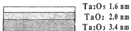
Figure 10. The structure of Ta-oxide/Ta multilayer based on the simulation for HRBS energy spectrum of Ta film after milling, specimen I.
